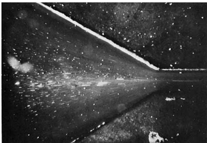
Fig. 3. Streak photograph of polystyrene melts at 200°C in a converging channel having a half-angle of 30 degrees; Q = 8.44 cc/min.
